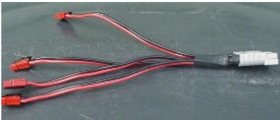
The connectors come in several sizes from 15 amps on up to 175 amps. I use 50 amp connectors for my power supply and 30 amp connectors on all the radio cables. Here is the photo of my 50 amp power buss for my power supply. It consists of a Anderson Gray SB Series 50 amp Powerpole connector with four 30 amp pigtails for connection to my radio equipment. My radios each have a 30 amp connector
